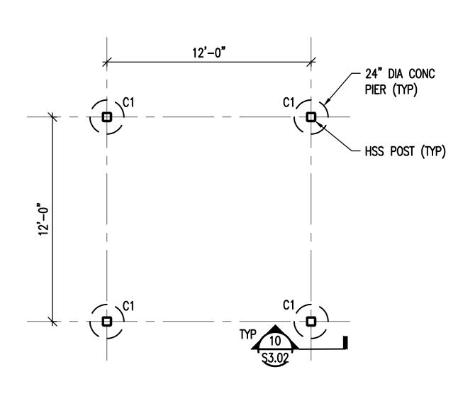
MECHANICAL PLATFORM FOUNDATION PLAN
