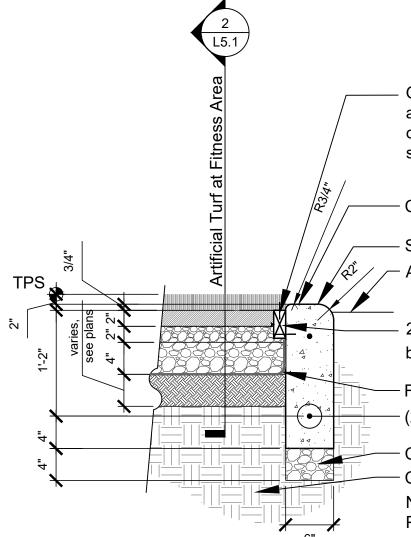
Glue nail board to sidewalk with outdoor adhesive pl premium polyurethane adhesive or equal. Fasten every 2' O.C. with concrete screws.
